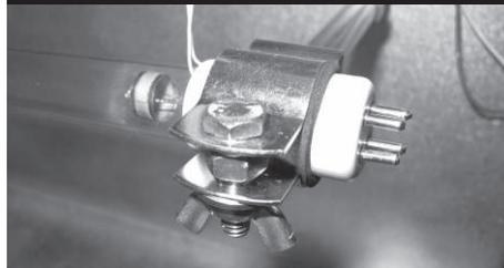
Insert the end-cap with foam gasket into the clamp assembly and tighten. Be careful not to over tighten as it may result in end-cap breaking.
