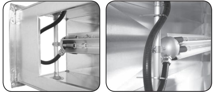
9.3 Connect the cable of the UV Bio-Wall Max to the ballast box. Pull the colored wire-set (20 wires) from the UV Bio-Wall Max into the ballast box through the knockout located between the 2 fans and secure the cable connector to the ballast box.
